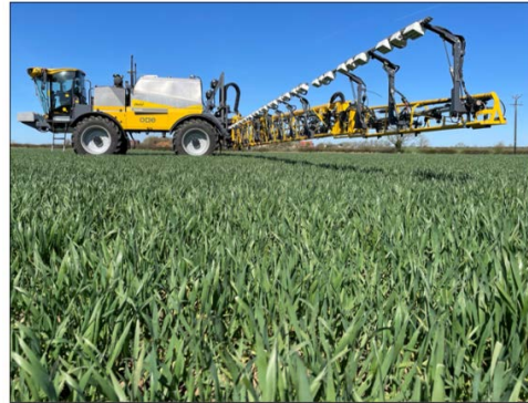
Chafer sprayer showing camera arrangement
